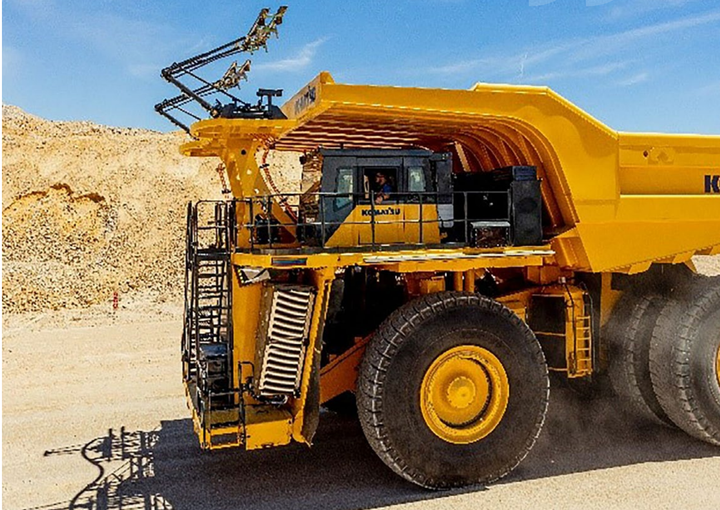
Fig. 4. Power-agnostic truck from Komatsu
